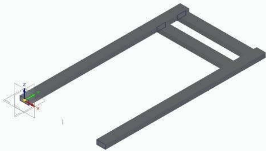
Fig. 5. Structural frame design of the hydrokinetic turbine showing the supporting arrangement.
