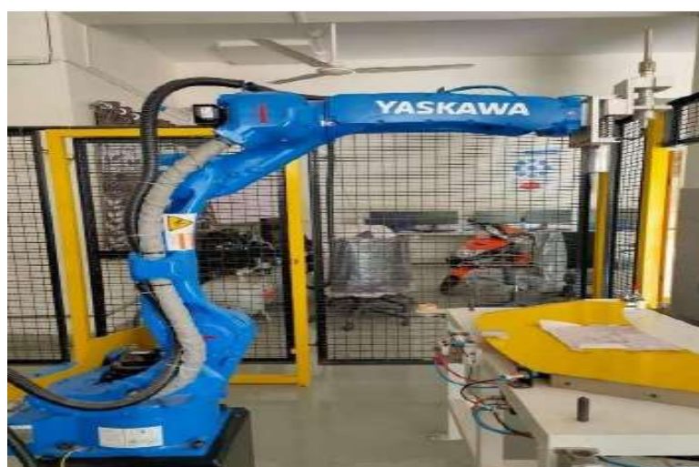
Figure 2: Ultrasonic welding robot setup.
